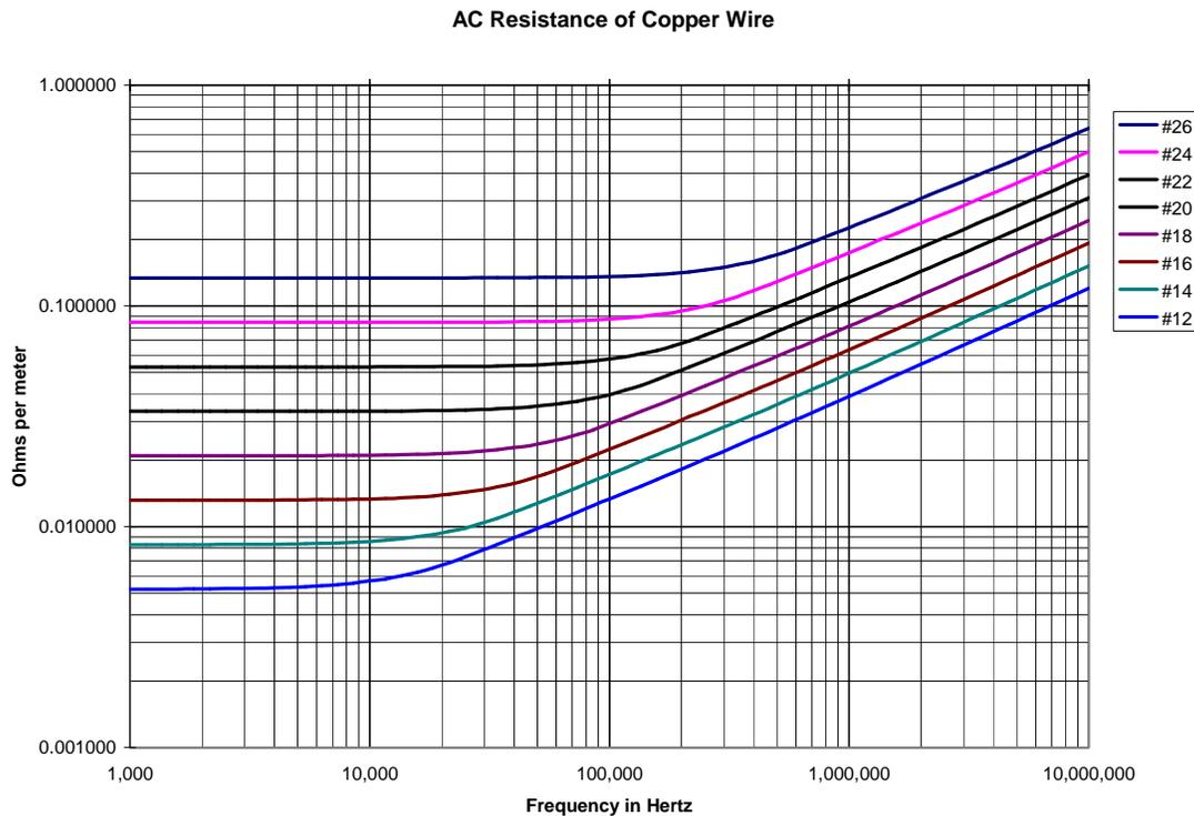
Figure 3: AC Resistance of Copper Wire
