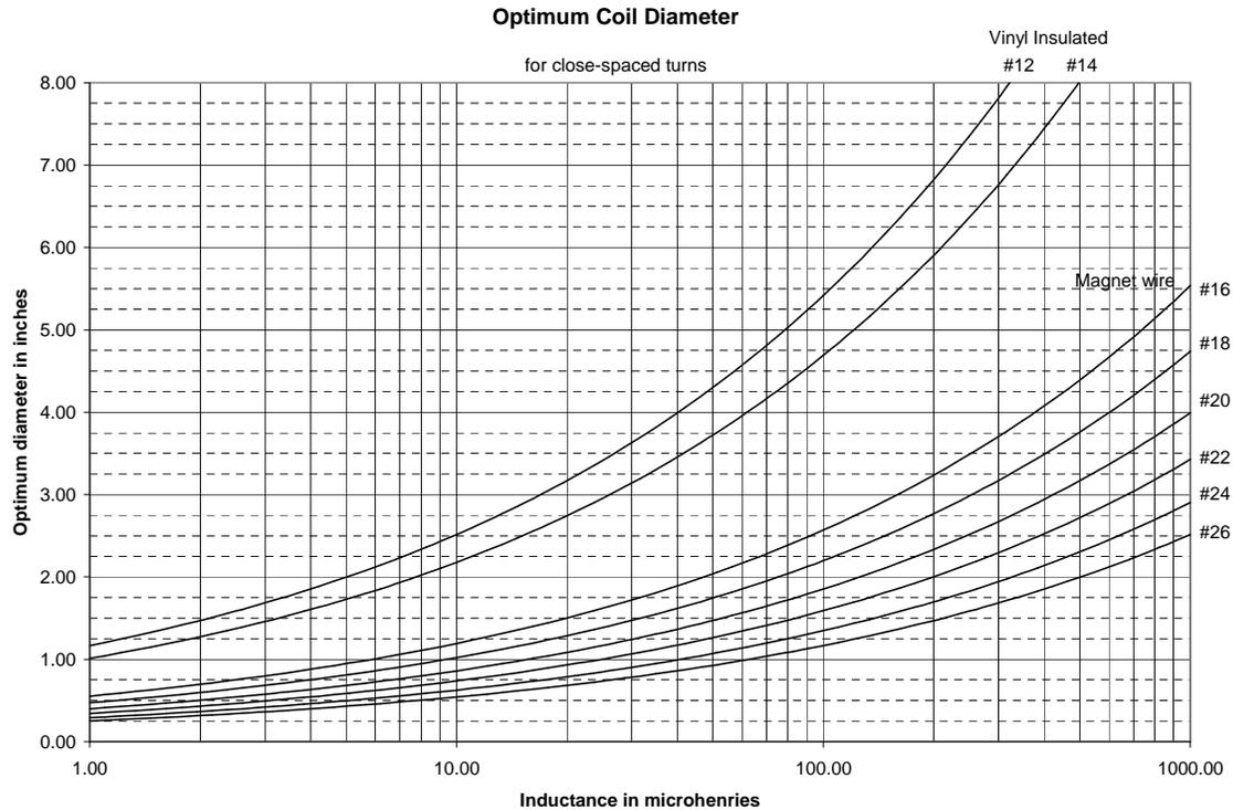
Figure 1: Optimum coil diameter
