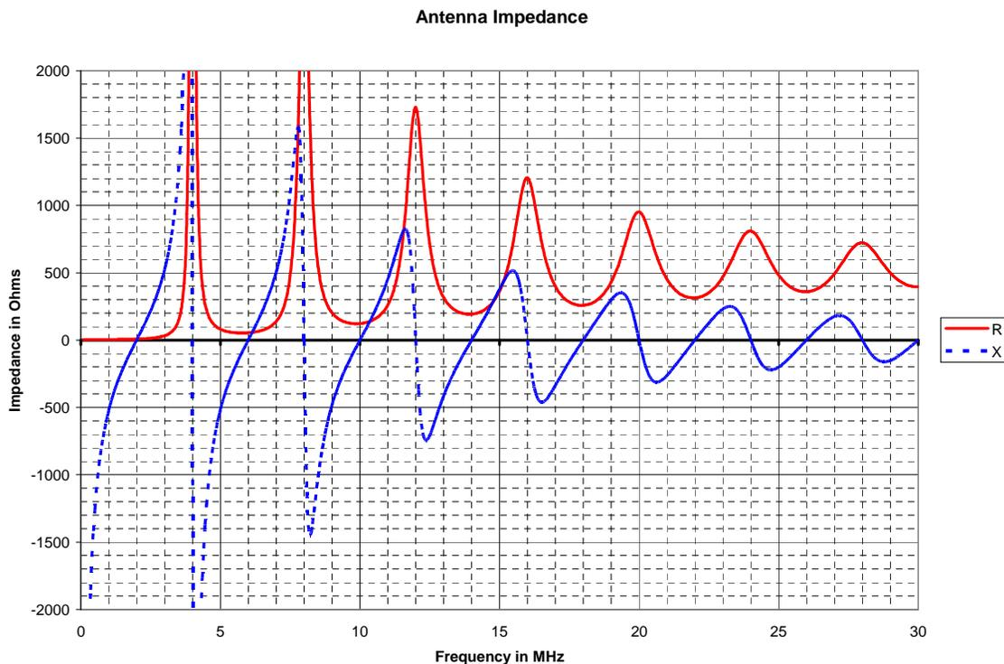
*Figure 3: 2 MHz resonate antenna 5 meters off ground*
