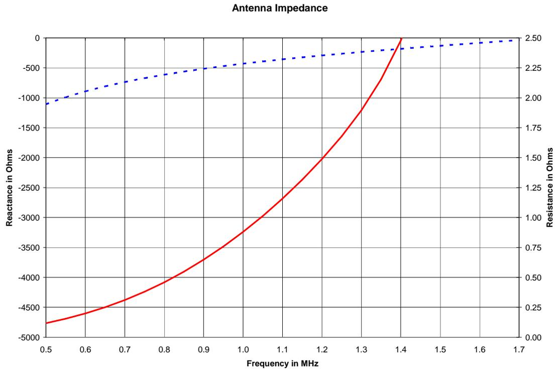
*Figure 7: Antenna length = 40 m, height = 5 m*
