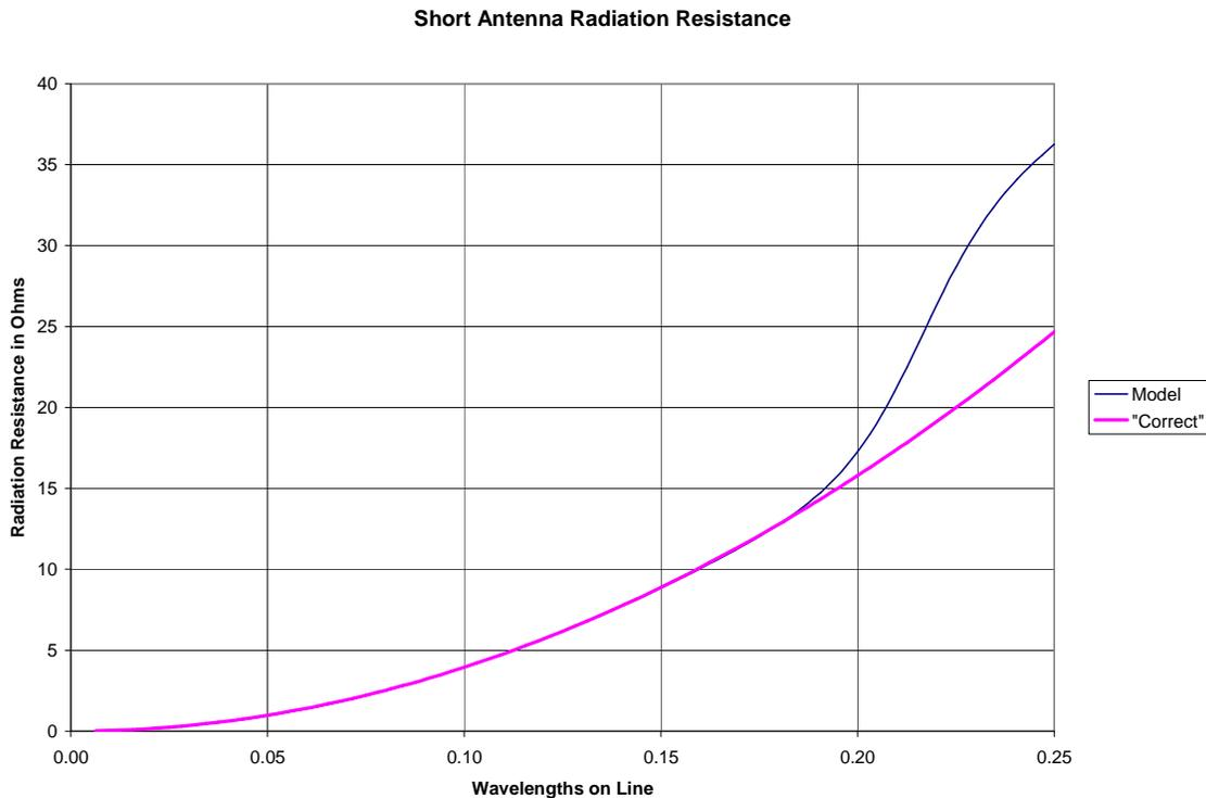
Figure 2: Model fit to short antenna radiation resistance
