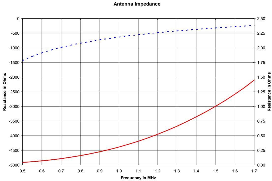
*Figure 6: Antenna length = 30 m, height = 3 m*
