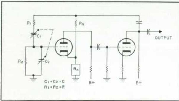
Figure 2. Basic Circuit of Resistance Capacity Oscillator
