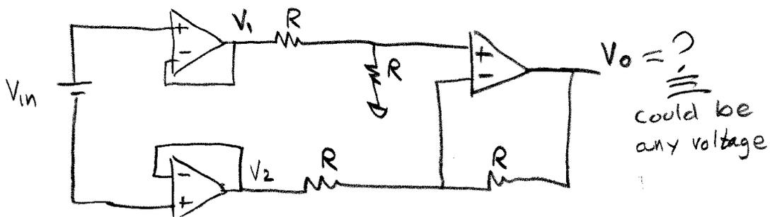
WE KNOW FROM PRIOR ANALYSIS THAT  $V_o = V_1 - V_2$ .
