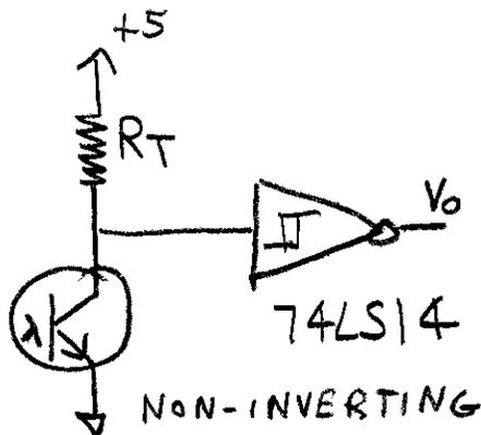
Figure 2: Binary light detector using logic Schmitt trigger
