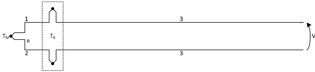
Figure 10: Failure to use thermocouple wire all the way. T_X is unknown.
