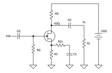
7. Complete the design of the following circuit.  $V_{DD}$  is +20 volts. The input resistance is to be 1 M. The drain current is to be 70% of  $I_{DSS}$ min. The load resistor is 470 Ohms,  $R^S$  is 1.8K and  $R_D$  is 680 Ohms. Av is to be -2.3 for a minimum  $I_{DSS}$  unit. Determine the required  $V_{GG}$  at the voltage divider formed by  $R_A$  and  $R_B$  (10K). Determine  $R_{S1}$  and  $R_A$ .
