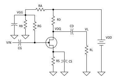
8. Complete the design of the following circuit.  $V_{DD}$  is +20 volts. The input resistance is to be 1 M. The drain current is to be 70% of  $I_{DSS}$ min. The load resistor is 470 Ohms. Determine  $R_S$ . Remember that problem 3 is the analysis of this.
