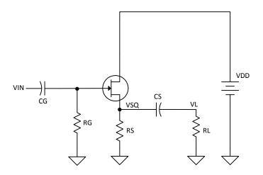
$V_{DD} = 20V$ ,  $R_S = 100$  Ohms,  $R_L = 470$  Ohms,  $R_G = 1$  M.
