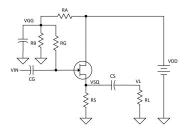
$V_{DD} = 20V$ ,  $R_S = 2.4$  K,  $R_L = 470$  Ohms,  $R_G = 1$  M,  $R_A = 51$  K,  $R_B = 10$  K.
