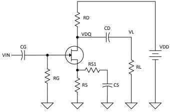
$V_{DD}=20$  volts,  $R_D=680,\,R_L=470,\,R_G=1M,\,R_S=1.8$  K,  $R_{S1}=22$   $R_A=75$  K,  $R_B=10$  K.
