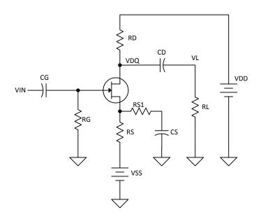
$V_{\rm DD}$  = 20V,  $V_{SS}$  =-2.5 V,  $R_S$  = 1.8 K,  $R_D$  =680 Ohms,  $R_L$  = 470 Ohms,  $R_G$  = 1 M,  $R_{S1}$  = 22 Ohms.
