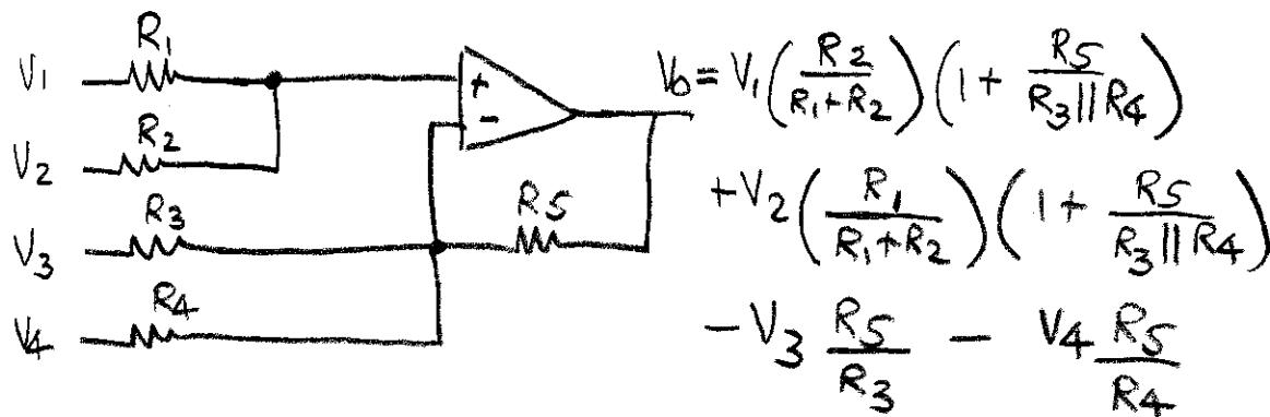
2. DETERMINE A SET OF RESISTORS TO IMPLEMENT THE FOLLOWING TRANSFER FUNCTION:
