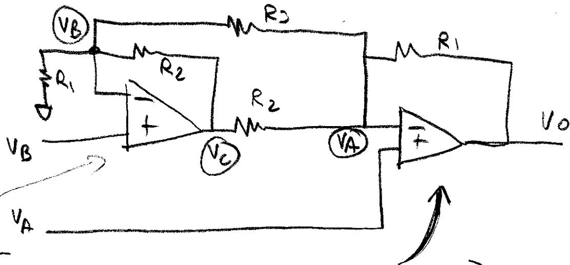
$$\left. \begin{aligned} \frac{V_C - V_A}{R_2} + \frac{V_B - V_A}{R_3} + \frac{V_O - V_A}{R_1} &= 0 \\ \frac{V_A - V_B}{R_2} + \frac{0 - V_B}{R_1} + \frac{V_C - V_B}{R_2} &= 0 \end{aligned} \right\} \text{THIS IS THE LONG WAY - BUT IT WORKS}$$
