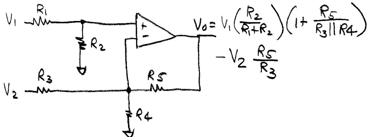
DERIVE THE DESIGN EQUATIONS FOR THIS CIRCUIT
